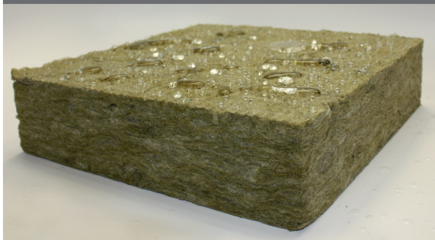
RainBarrier® HD is a high density board that provides thermal insulation, fire protection and acoustical control while efficiently draining water from a wall cavity system.
